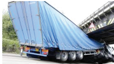
Figure 1: Hazard of insufficient information on suitable access routes for HGV drivers
