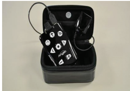
Figure 1: The world-unique hybrid GNSS for blind and visually impaired within its protective transport cover: the ANGIO Mobile device
