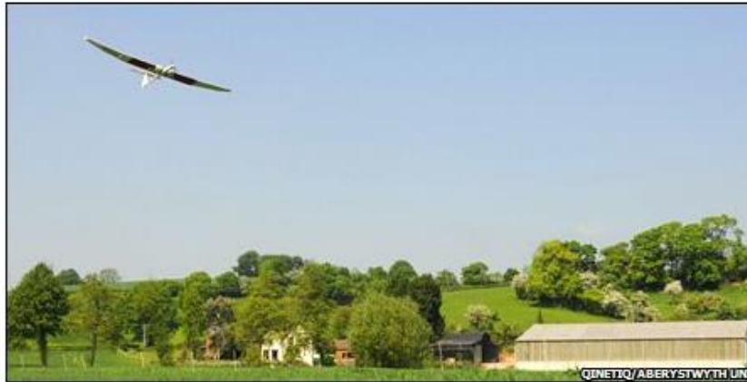
The robot plane can stay aloft for about an hour on battery power
