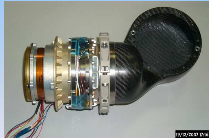
Dexarm Joint integrated with carbon fibre limb
