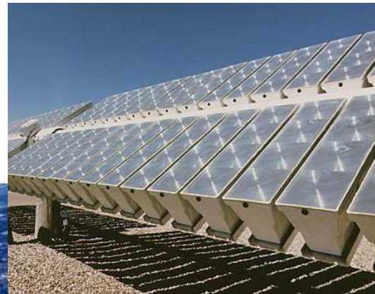
Fresnel solar concentrator
